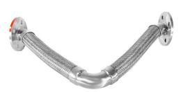
As opposed to bellows expansion joints, Kanwal's Easyflex Series Flexible "EFSVC" Connectors impose no pressure thrust load on the piping system, eliminating the need for thrust anchoring around the connector. Simply use pipe alignment guides in conjunction with the seismic "EFSVC" connectors to direct any motion into the connector.
