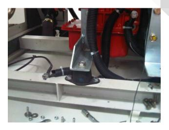
EFTM rubber mountings are designed to provide superior attenuation of medium to high frequency vibration and noise emanating from a wide range of motor driven machines particularly axial and centrifugal fans. High resilence rubber with low dynamic to static stiffness ratio ensures maximum efficiency, good creep performance and long service life.
