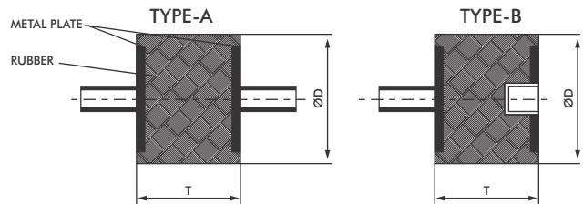
**Easyflex** Type EFRO mounts are very versatile and can be ideal for a wide range of applications where simple and compact anti-vibration mountings are required. They are suitable for loads in shear, as well as in compression. These mounts are used in an extensive range of applications including compressors, generators, air conditioners, pumps, fans, motors, laboratory equipment, scales, etc.
